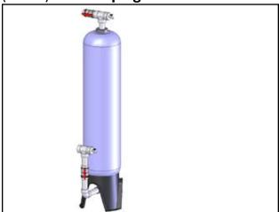
Connect the inlet and outlet plumbing according to your preferences and any applicable local codes. Include sample/drain ports with hose bibb connections on inlet and outlet piping to facilitate startup and service.
