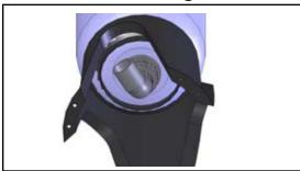
Connect the Union fitting to the inlet bushing
