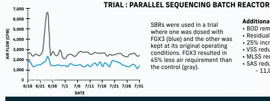
SBRs were used in a trial where one was dosed with FGX3 (blue) and the other was kept at its original operating conditions. FGX3 resulted in 45% less air requirement than the control (gray).
